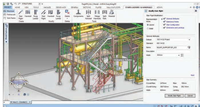
The Stairs, Ladders & Handrails application, showing stair design (above) and ladder design (below)
